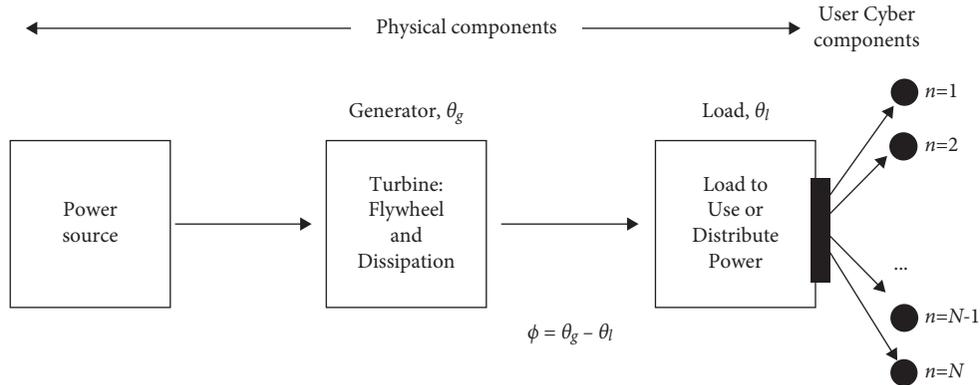
FIGURE 3: An electric grid consisting of one generator (with rotor angle  $\theta_g$ ) and one load (with rotor angle  $\theta_l$ ), in this case envisioned as a utility company that has  $N$  consumers, indexed by  $n = 1, 2, 3, \dots, N$ , with AMI. Our analysis focuses on the consequences of compromise of the AMI rather than attacks on the cyber system of the power generating system.
