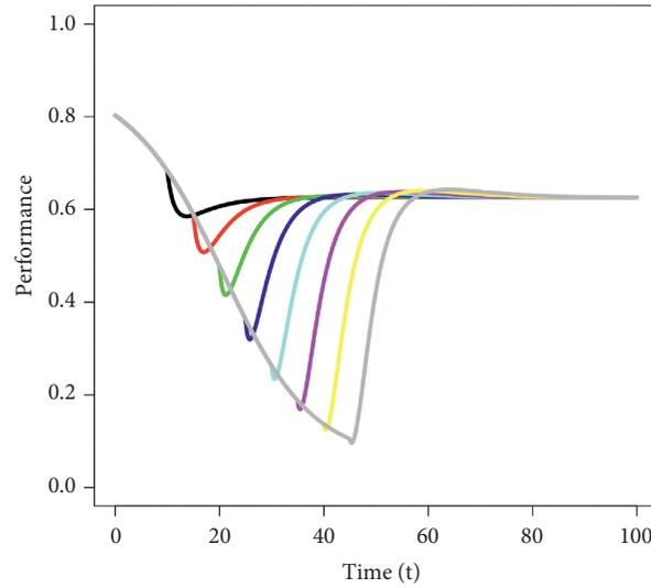
FIGURE 6: Performance of the physical system for the detection times in Figure 5. Although in all cases performance reaches the same steady state (about 70% of performance before compromise and activation of DCM), minimum performance varies considerably according to the time of detection of compromise.
