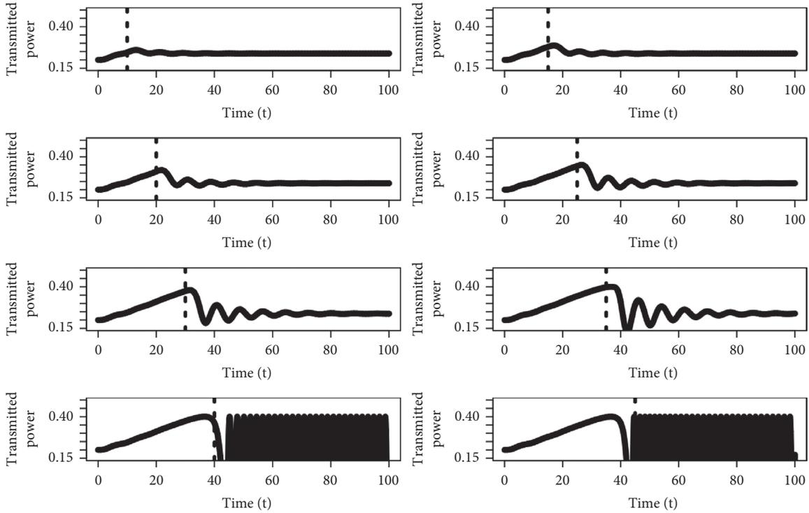
FIGURE 9: Transmitted power when the model for the grid and compromise are connected by assuming that  $P_0$  in equation (16) is replaced by  $P_0(1 + \varepsilon_d y(t))$  with  $\varepsilon_d = 0.04$  representing how much one compromised AMI increases the demand for power, and  $y(t)$  is the number of compromised cyber components. The dynamics of compromise and times of detection are the same as in shown in Figure 5—the vertical dotted line denotes the time at which compromise is detected.
