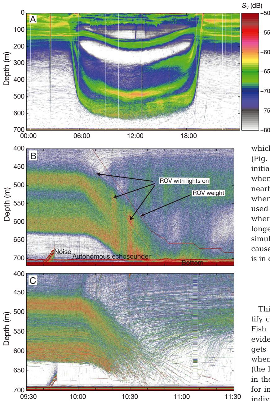
Fig. 1. (A) Diel echogram (20 May 2015). (B,C) Manipulating the vertical distribution of mesopelagic scattering layers using a remotely operated vehicle (ROV) with artificial light. (B) Echogram (38 kHz) from the ship operating the ROV (depicted in the echogram). (C) Simultaneous echogram (38 kHz) from an upward-looking autonomous echosounder located at the bottom. Color scale refers to volume backscatter ( $S_v$ ), a proxy for abundance
